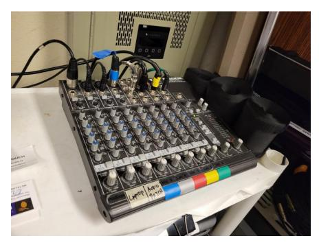
The far left set of control knobs is for the podium levels. Do not change any of the lower knobs. All are at the 12:00 position.
