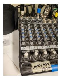
If you need to change the mic level of the podium mic or the separate mic for the CuH room, use the knobs labled "TRIM" to change the gain.
