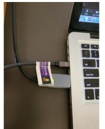
HDMI video connector on top. USB audio on bottom with green light.
